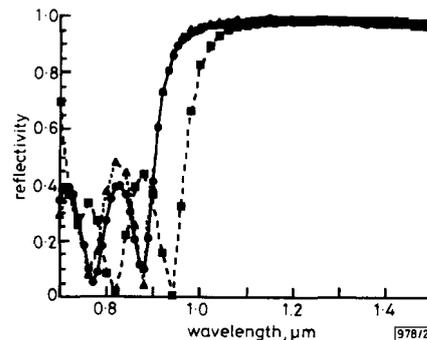
Fig. 2 Measured reflectivity spectra of mirror with three stack plus cap oxide layer
