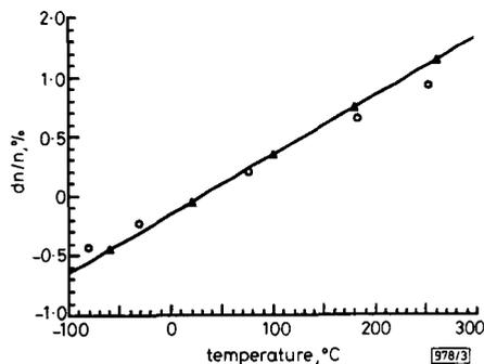
Fig. 3 Variation of refractive index with temperature
