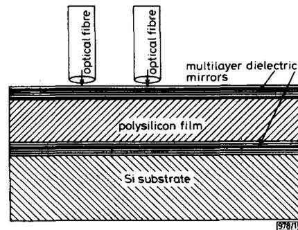
Fig. 1 Device layout and geometry
