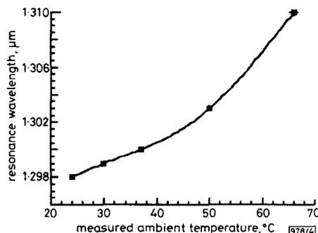
Fig. 4 Temperature dependence of resonance wavelength
