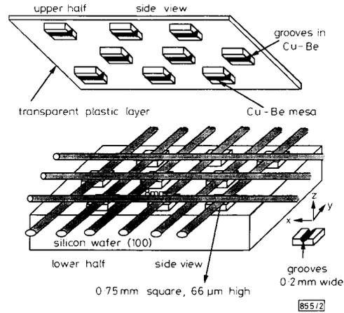
Fig. 2 Fabricated sensor structure
