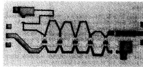
Fig. 2 5-45 GHz monolithic InP HEMT distributed amplifier
