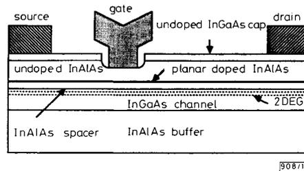
Fig. 1 Cross-section of InP HEMT
