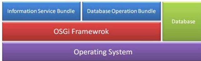
Fig. 3. Service provider server OSGi architecture.
