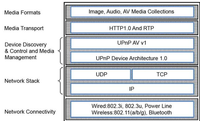
Fig. 1. DLNA transmission architecture.
