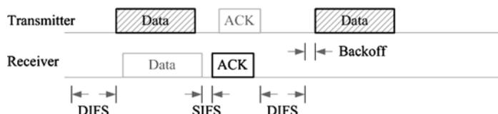
**Fig. 2** Virtual carrier sensing mechanism in DCF
