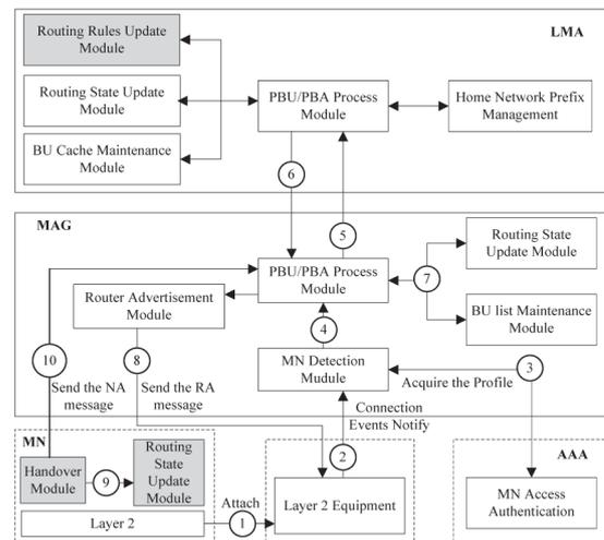
Figure 3 Implementation Modules of PMIPv6 and Its Multihoming Extension
