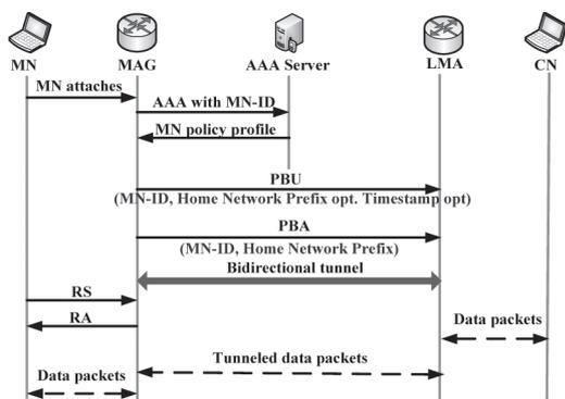
Figure 1 Signaling Call Flow of Basic PMIPv6
