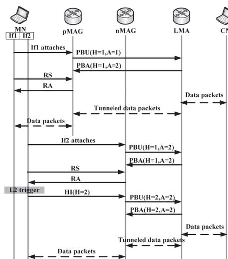
Figure 2 Signaling Call Flow of Multihoming PMIPv6
