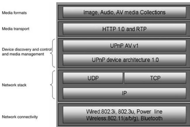
FIGURE 1. The DLNA transmission architecture.
