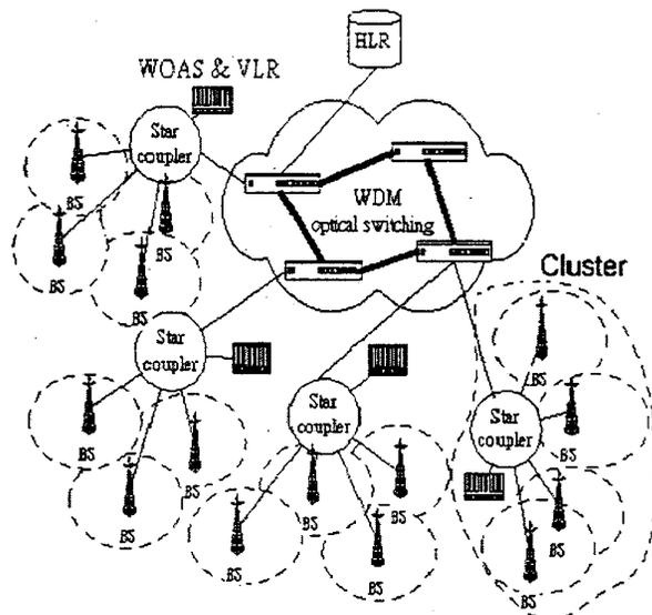
Fig. 1. WDM-based PCN architecture
