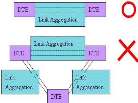
Figure 1 Multi-node connection will have the loop problem
