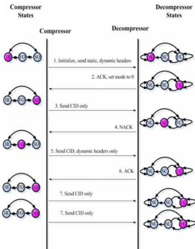
Figure 4 Finite state machines of RoHC Trunk
