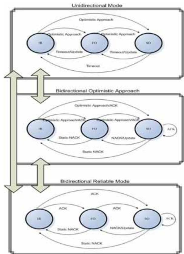
Figure 5 Finite state machines for the ROHC compressor/decompressor
