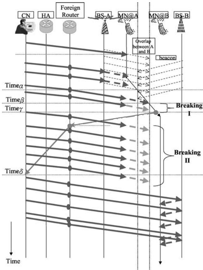
Figure 3. Timing diagram during handoff in Mobile IPv6 scheme.
