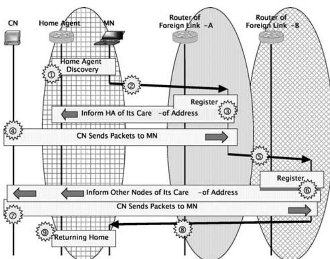
Figure 1. Overview of the IETF Mobile IPv6.
