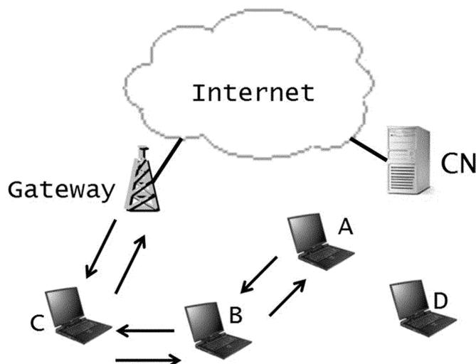
Fig. 3. Mobile *ad-hoc* network where A is communicating with the gateway to the Internet through B and C; CN is correspondent node [4].
