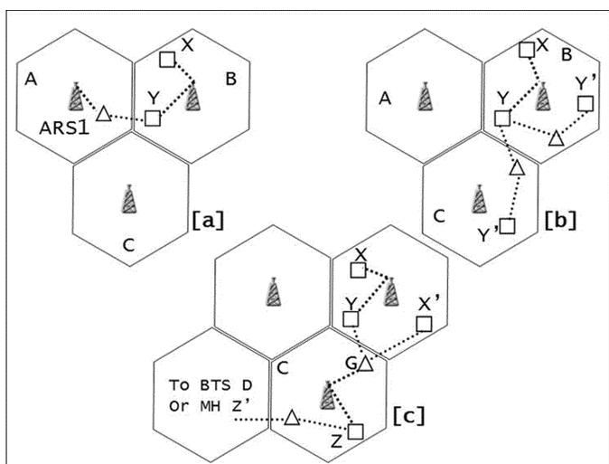
Fig. 2. An integrated cellular and *ad-hoc* relay system [3].
