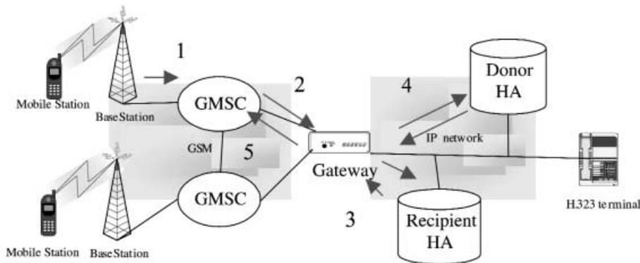
Figure 2. IPv6-GSM GSM (NP) registration
