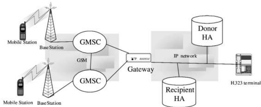
Figure 1. IPv6-GSM network architecture
