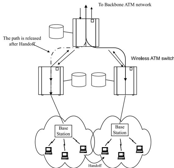
Fig. 1. A cell architecture in wireless ATM network.
