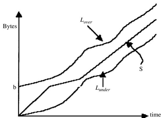
Figure 1. Basis of the smoothing plan
