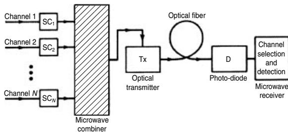
Fig. 4. A multichannel SCM light system.
