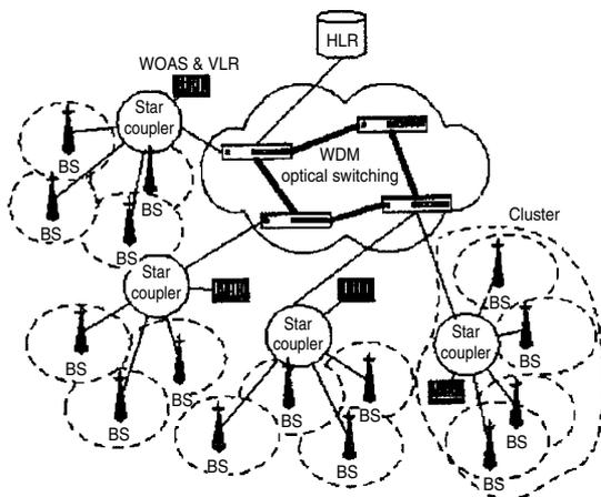
Fig. 1. WDM-based PCN architecture.
