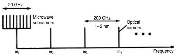
Fig. 5. Frequency allocation in a multi-wavelength SCM network.
