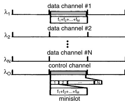
Fig. 2. Data and control channel formats.
